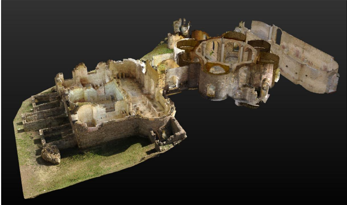
Fig. 13. Overall 3D model of the Villa's bath complex generated by terrestrial laser scanning.
