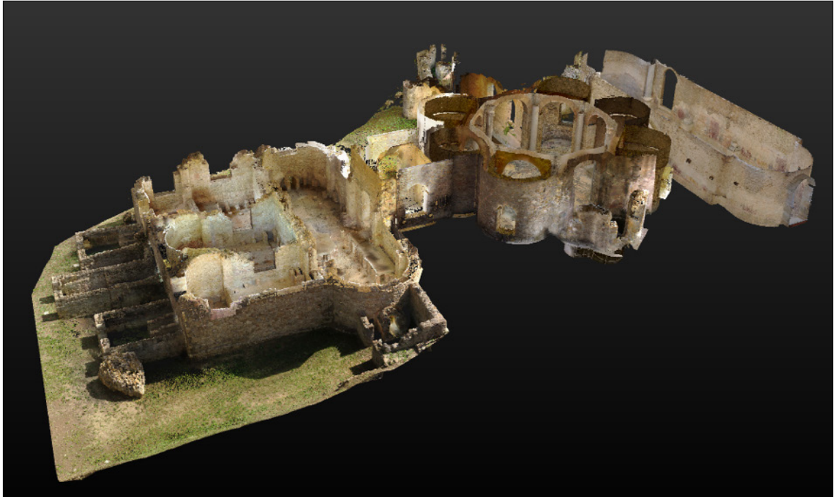
Fig. 13. Overall 3D model of the interior and exterior of the Villa's bath complex generated by terrestrial laser scanning.
