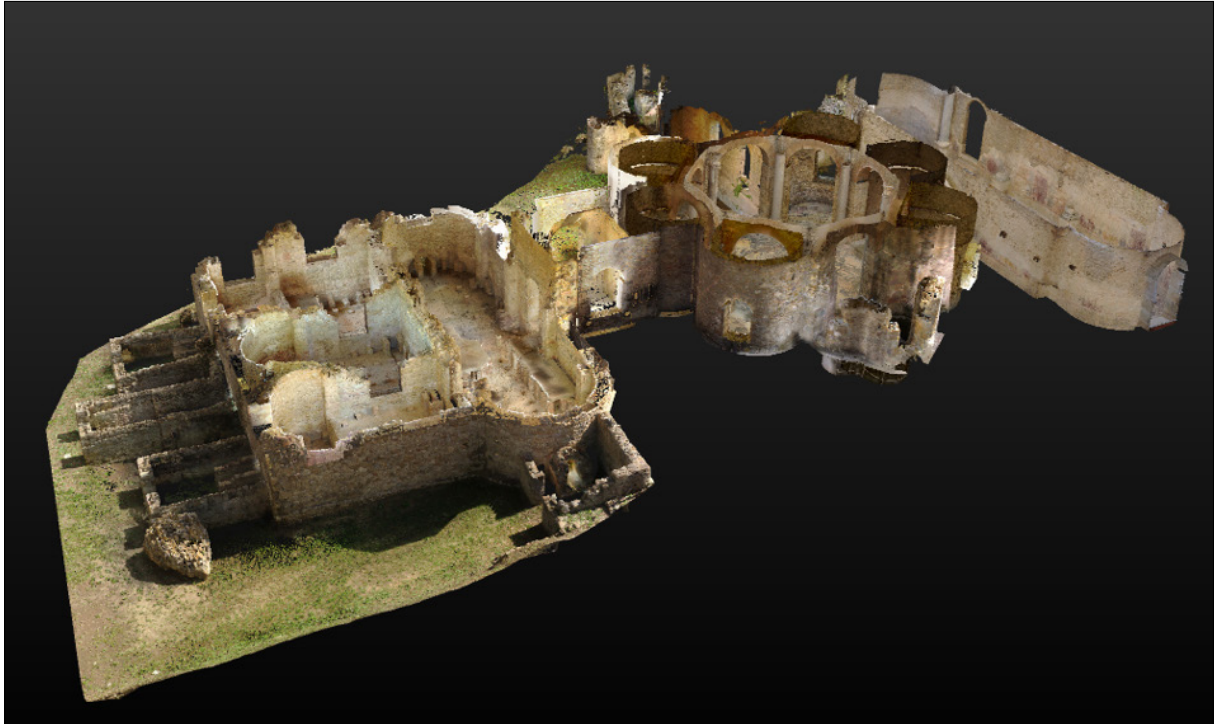
Fig. 13. Overall 3D model of the Villa's bath complex generated by terrestrial laser scanning.
