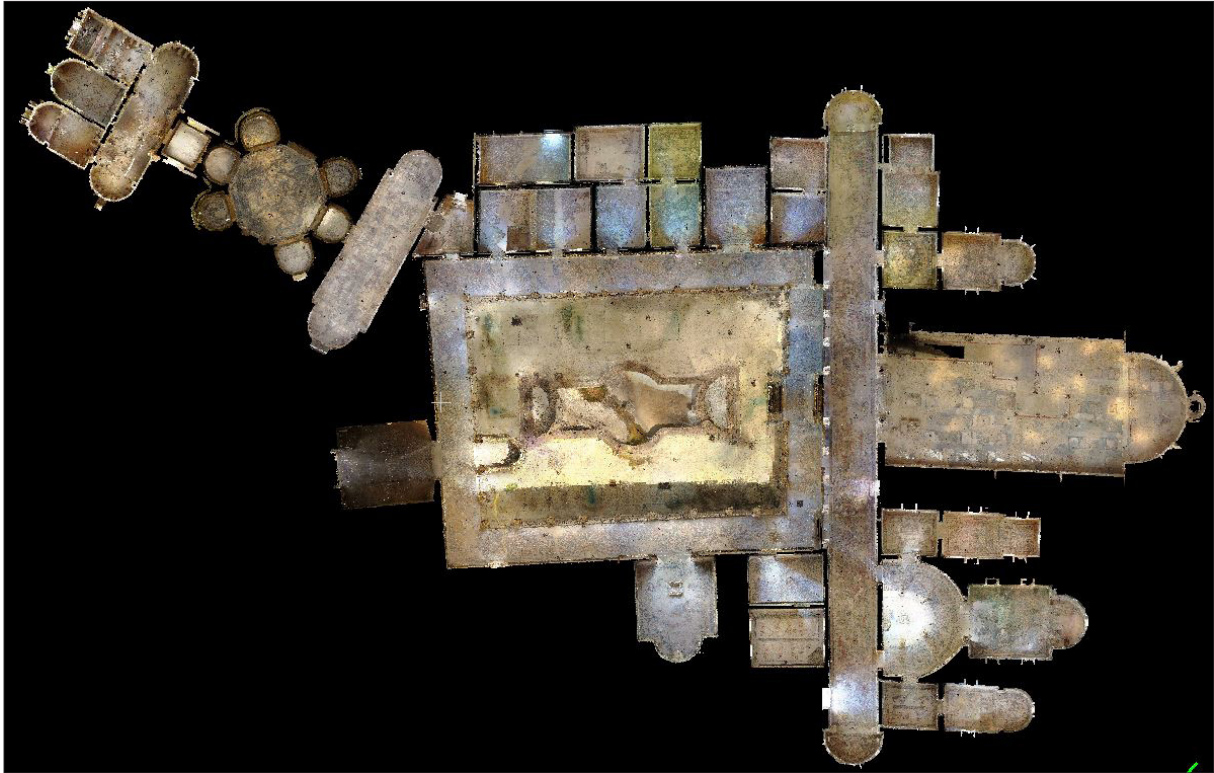
Fig. 1. 3D colored point cloud of the interior of the Villa generated by terrestrial laser scanning.
