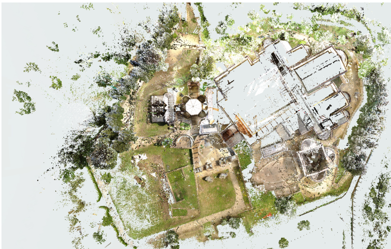
Fig. 6. 3D colored point cloud of the exterior of the Villa generated by terrestrial laser scanning.
